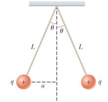
Two identical small charged spheres, each having a mass of  $3 \times 10^{-2} \, kg$  hang in equilibrium as shown. The length (L) of each string is 0.150 m, and the angle  $\theta = 5^{\circ}$  . Find the magnitude of the charge on each sphere.
